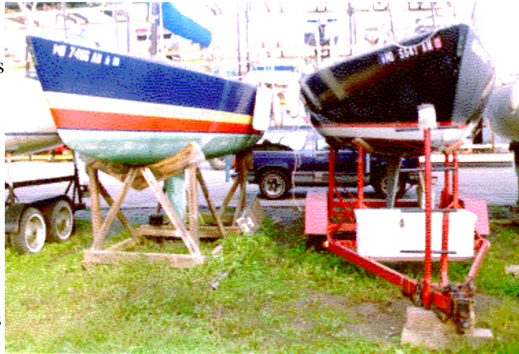
You must decide how important a trailer is to you. In this yard, boats are launched with a huge forklift. Here, a wooden cradle is great for a local racer, but just try to hit the road with that cradle.
